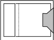
All measurements are internal and in millimeters. 18 mm material is recommended throughout. Butt joints can be used but all joints must be airtight.
